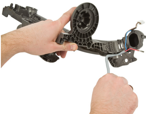
135 Remove the internal powercord assembly from the duct assembly.
